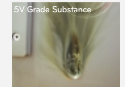
Fire is extinguished as soon as the naked flame is removed
